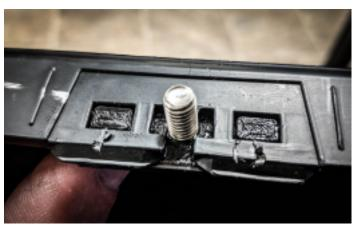
7.) Apply a medium strength thread locker and tighten all bolts with a 4mm allen socket. Be careful not to over tighten the bolts going through the Fender Retention Washers. This completes Step 2.
