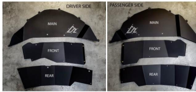
2.) Using (8) M6 x 12mm Button Head bolts and a 4mm allen socket, assemble the three panels into a unit. Leave these bolts loose until final assembly. The assembly should look like the images below. (Passenger side pictured)
